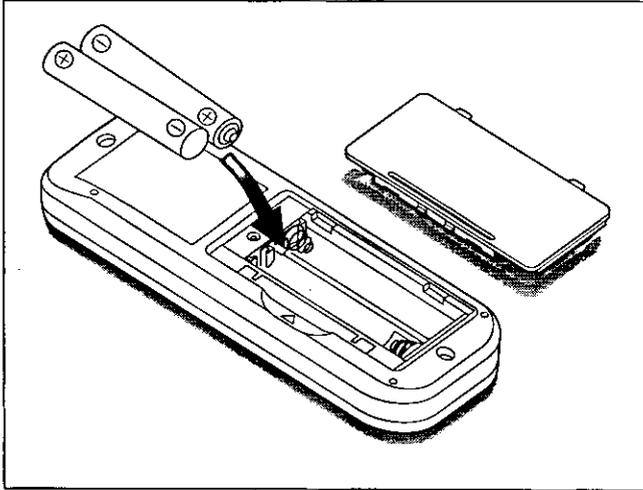
To remove the batteries, pull out the  $\oplus$  side.
