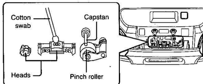
It is recommended that the head assembly be demagnetized if distortion or poor sound quality persists after cleaning the heads. Demagnetize them using a demagnetizer available from an audio store.
