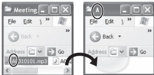
Reload the files to the original folder that the files were imported from. When you reload the files to other folders, those files cannot be played on this unit. (Confirm the first character (A to D) of the file name matches the folder name (A to D).)
