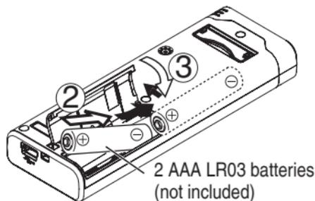
Make sure the batteries face the right direction.
