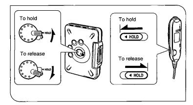
This function prevents the unit from operating even if one of the buttons is pressed in error.
