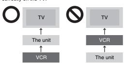
When connecting the unit to a TV with a built-in VCR, connect to the input terminals on the TV, not the VCR.
