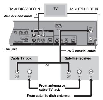
You can record and view scrambled and unscrambled channels simultaneously if connections are made as shown in the diagram below.
