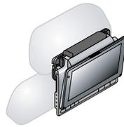
Use the monitor in the open position as shown in the illustration to the right to prevent abnormal audio or damage resulting from vibrations in the car. The angle of the monitor can be adjusted up to about 30°.
