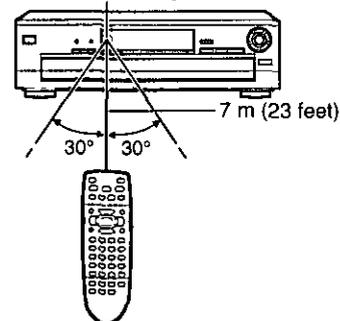
Aim at the sensor, avoiding obstacles, at a maximum range of 7 m (23 feet) directly in front of the unit.
