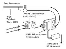
• If your television has both lead and coaxial VHF terminals, use the lead connection to minimize signal loss.
