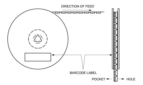
Figure 8. Reel Winding Direction
