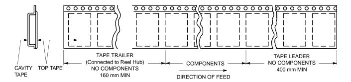
Figure 5. Tape Ends for Finished Goods
