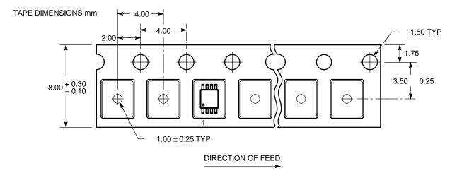
Figure 6. US8 Reel Configuration/Orientation
