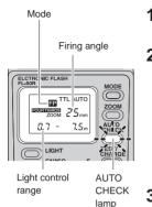
**1** The control panel shows the light control range according to the camera's setup.
