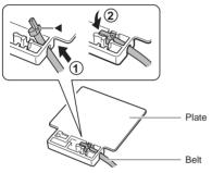
**2** Align the flat surface of the plate with the electronic flash and wrap the belt around the flash (1). Insert the other end of the belt firmly into the plate (2).
