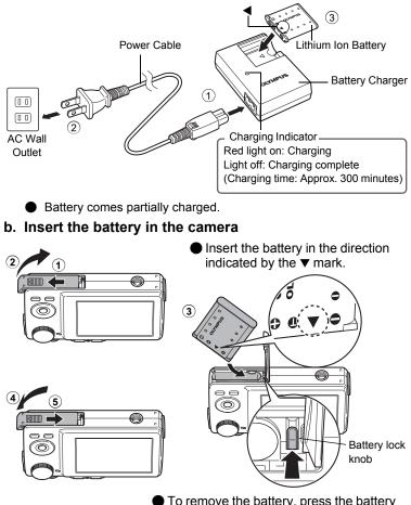
To remove the battery, press the battery lock knob in the direction of the arrow.
