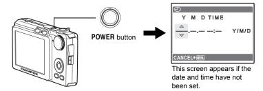
• To turn off the camera, press the **POWER** button again.
