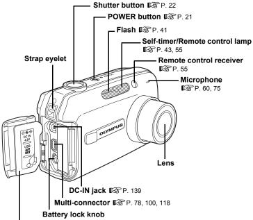
Battery compartment/Connector cover P. 78, 118
