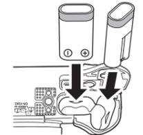
The correct way to insert the AA batteries is indicated on the bottom of the camera.
