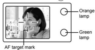
3 Press the shutter button gently (halfway) to adjust the focus.
