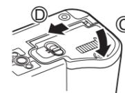
6 Slide the battery compartment lock from ⊕ to ⊖.
