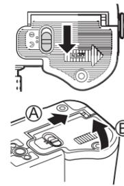
4 Insert the batteries, making sure that they are correctly oriented as shown in the illustration.
