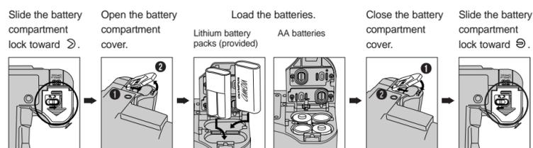
\* Close the battery compartment cover while pressing the batteries with the cover.
