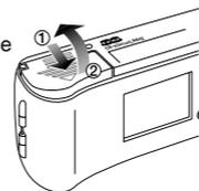
3. Insert the battery in the direction shown in the figure.
