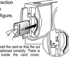
Be sure to hold the card so that the cut corner is positioned correctly. There is an arrow inside the card cover, indicating the insertion direction.
