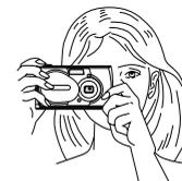
3. Press the shutter button halfway (half-press) to make sure the green lamp on the right of the viewfinder lights.
