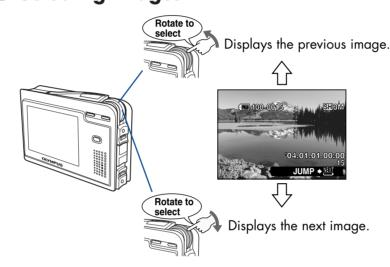
Pressing **BACK/NEXT** switches the playback method between the one-by-one mode and the 10-frame jump mode.
