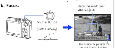
can be taken is displayed. The green lamp indicates the focus and exposure are locked.
