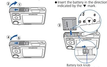
To remove the battery, press the battery lock knob in the direction of the arrow.
