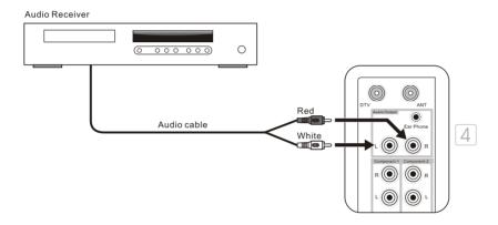
**Note:** When connecting an Audio output signal, an external Audio amplifier is necessary to amplify the signal for external speakers.
