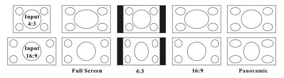
Full Screen Enlarges the picture to 16:9 wide mode, by stretching the picture horizontally only.
