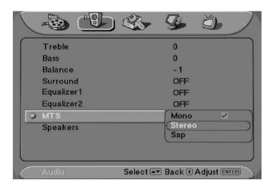
Additionally, you can press the hotkey "MTS" until the desired sound in dication appears. Each time you press the button, the sound indication changes as follows:
