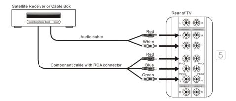
**Note:** The Y, Pb and Pr jacks do not provide audio, so audio cables must be connected to provide sound.
