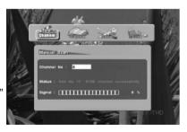
for aligning the direction of the antenna to improve the signal.
