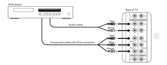
**Note:** The Y, Pb and Pr jacks do not provide audio, so audio cables must be connected to provide sound.
