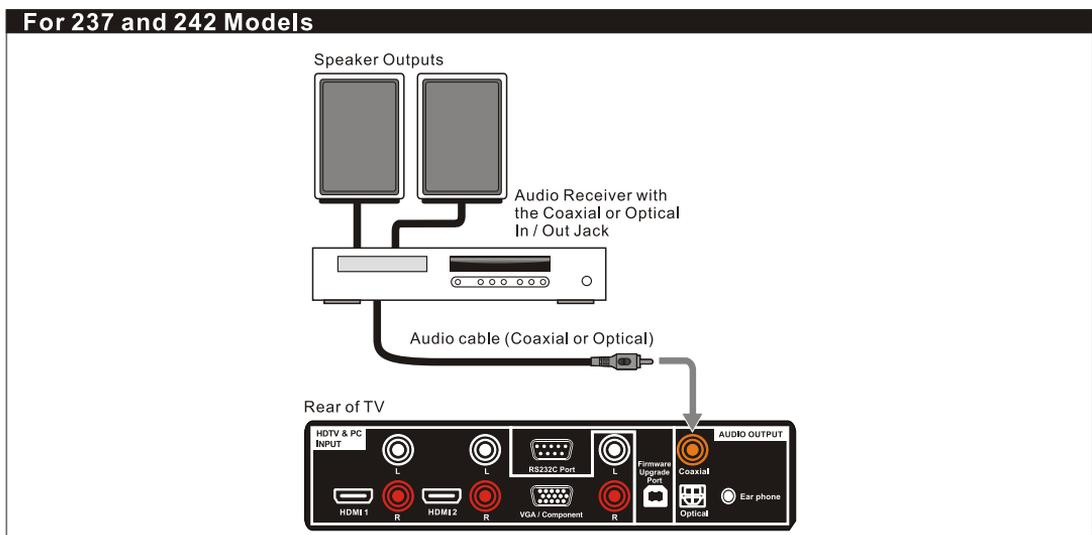
**Note:** Speakers must be amplified using an audio receiver such as a Home Theater System to amplify the audio from the TV.
