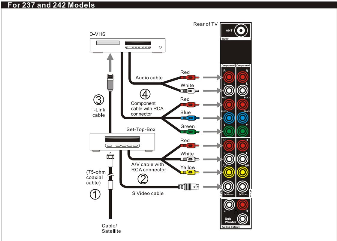
**Note:** The Y, Pb and Pr jacks do not provide audio, so audio cables must be connected to provide sound.
