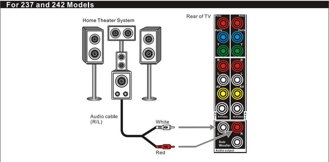
**Note:** When connecting an Audio output signal, an external Audio amplifier is necessary to amplify the signal for external speakers.
