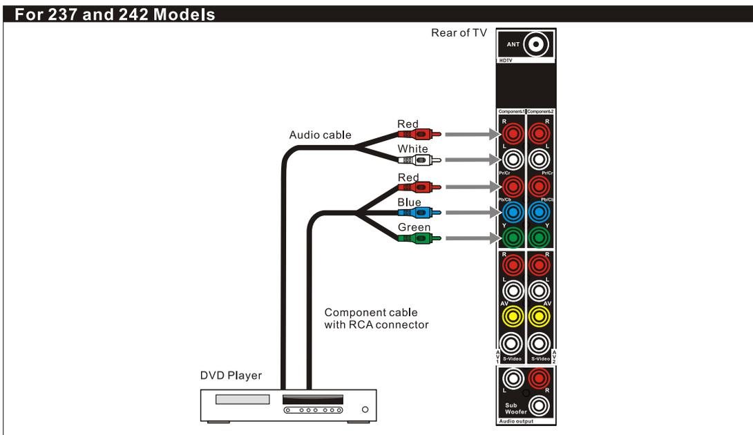
**Note:** The Y, Pb and Pr jacks do not provide audio, so audio cables must be connected to provide sound.
