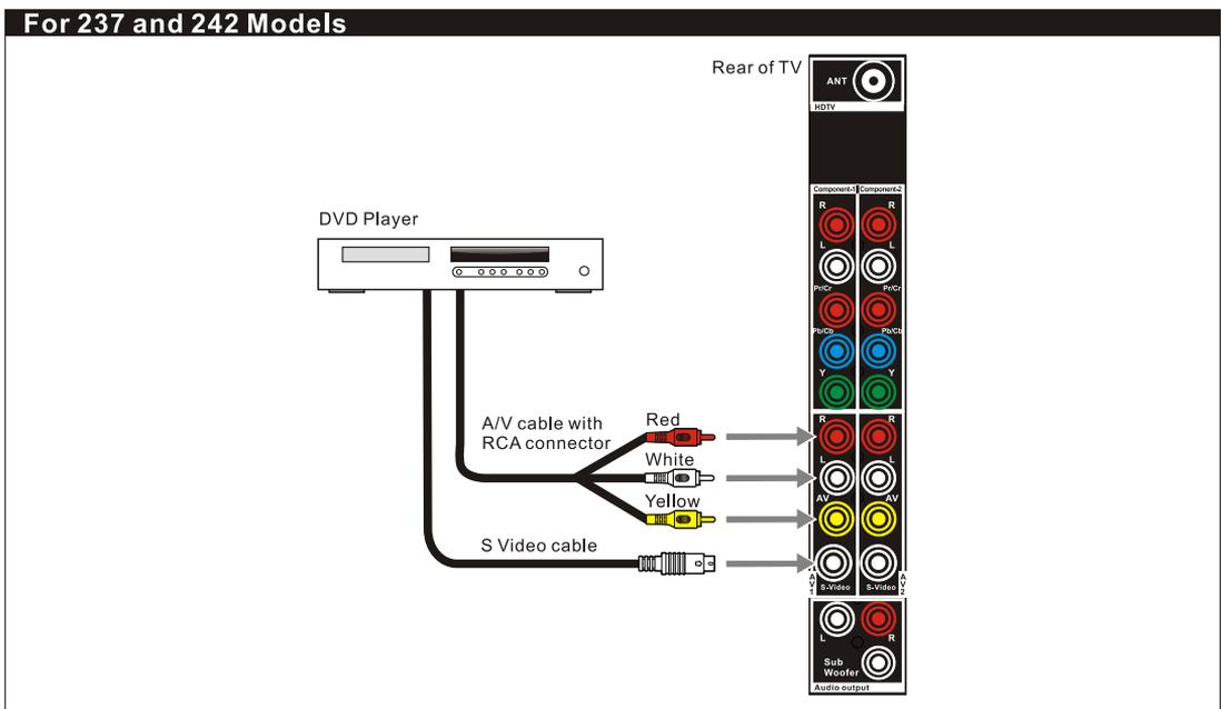
**Note:** When you connect video equipment to both the same Video and S-Video input jacks, the display will automatically select S-Video first.
