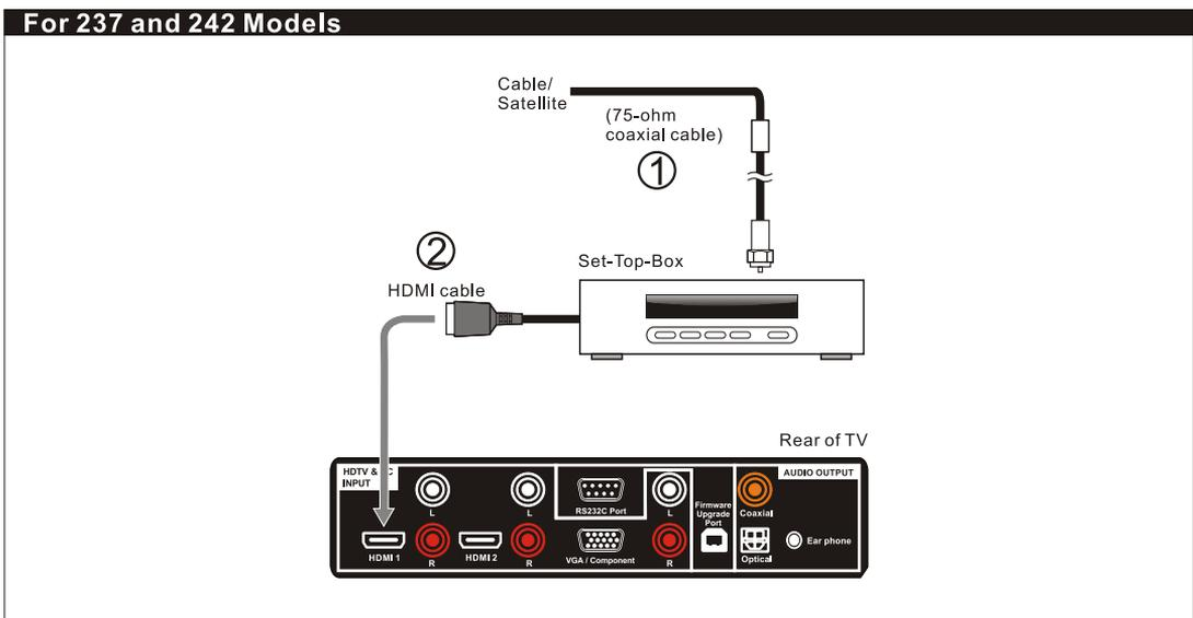
**Note:** HDCP is a copy protected digital connection that receives analog or digital video and audio signals from equipment with a HDMI output that features the HDCP function. HDMI allows the transfer of digital uncompressed data to the TV. This connection is superior when compared to the Component, S Video or AV (composite) connections.
