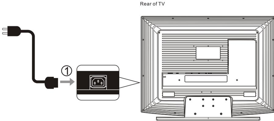
2. Connect the other end of the power cord to the wall outlet.
