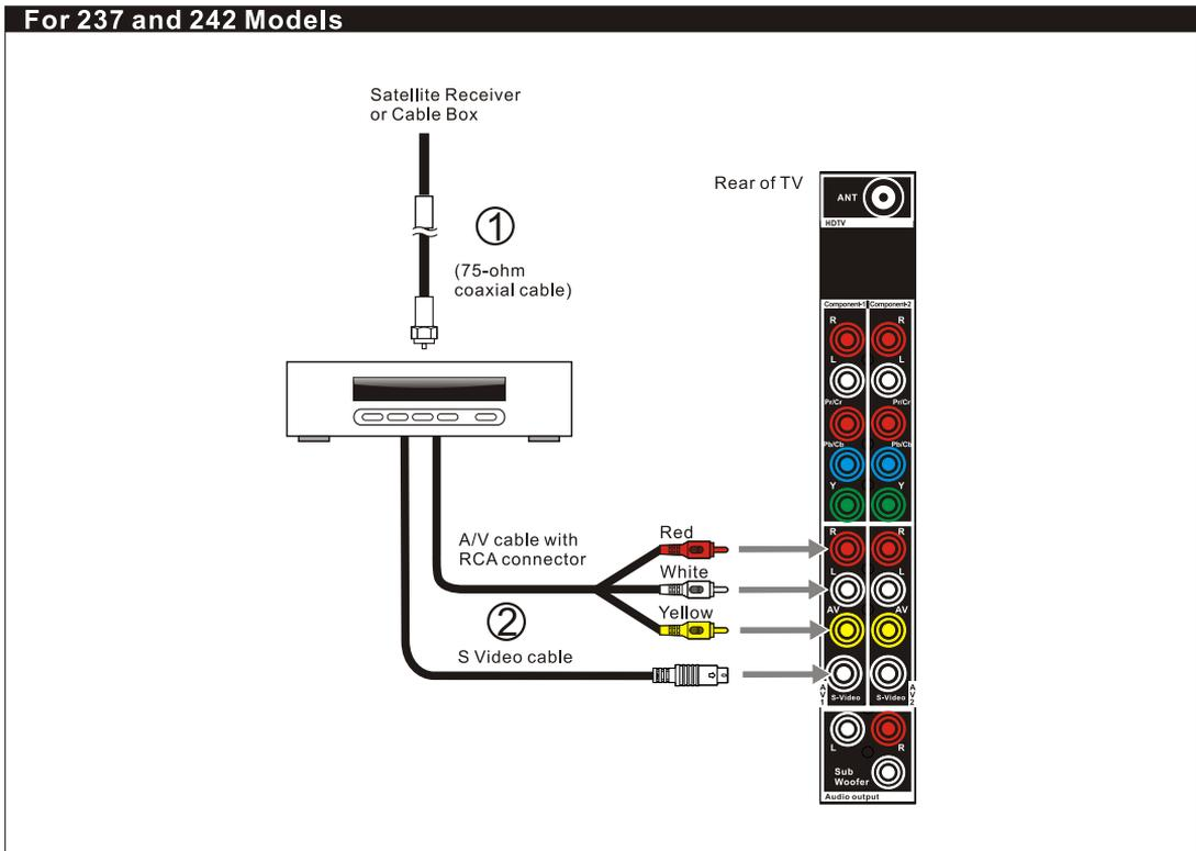
**Note:** When you connect video equipment to both the same Video and S-Video input jacks, display will automatically select S Video first.
