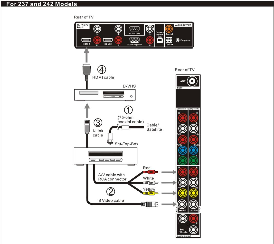
**Note:** HDCP is a copy protected digital connection that receives analog or digital video and audio signals from equipment with a HDMI output that features the HDCP function. HDMI allows the transfer of digital uncompressed data to the TV. This connection is superior when compared to the Component, S Video or AV (composite) connections.
