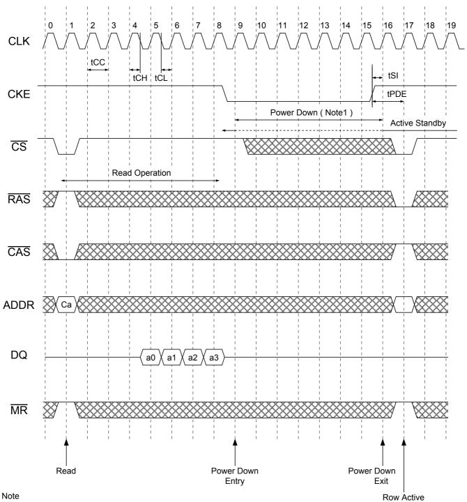
Minimum current consumption is expected in Power Down state. Low level CKE sampled only in Active Standby state is defined as Power Down "Entry" command and it cuts current consumption into minimum level. After Power Down "Exit" the contents of Mode Register and row address is preserved. During Power Down state no command can be sampled. Mode Register Set @ CAS Latency = 4, Burst Length = 4
