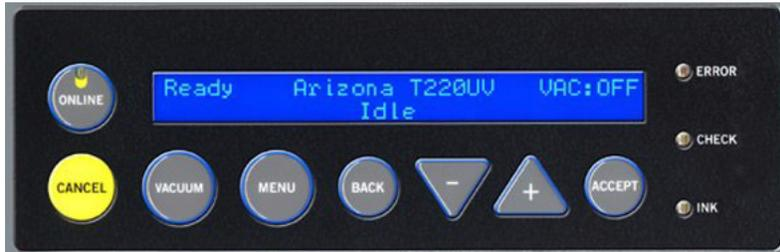
[35] Key Pad, Display Screen, and Status LEDs
