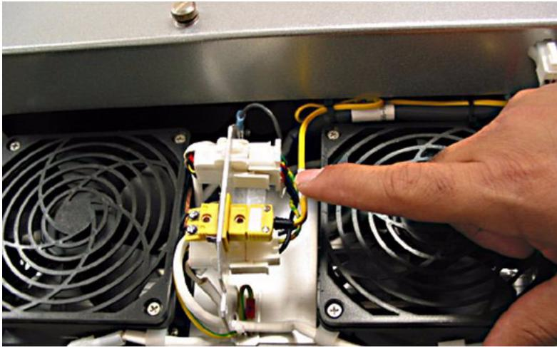
[75] Cable, Sensor and Power Connectors
