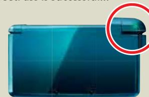
The Wireless LED illuminates when wireless communication is activated.
