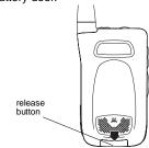
**3** Allow the battery door to pop up, slide it forward, and remove it from the back of your phone.
