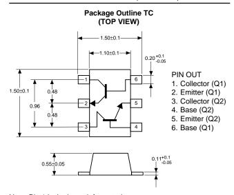
Note: Pin 1 is the lower left most pin as the package lettering is oriented and read left to right.
