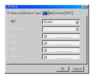
Select this option whether using the WEP (Wired Equivalent Privacy) key for encryption or not. To use encryption, specify WEP key.
