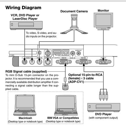
NOTE: When using with a notebook PC, be sure to connect between the projector and the notebook PC before turning on the power to the notebook PC. In most cases signal cannot be output from RGB output unless the notebook PC is turned on after connecting with the projector.
