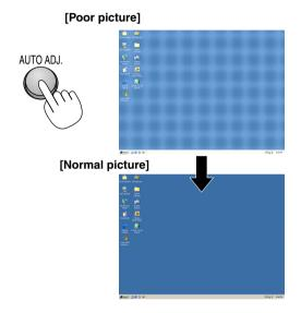
Press the Auto Adjust button to fine-tune the computer image or to remove any vertical banding that might appear and to reduce video noise, dot interference or cross talk (this is evident when part of your image appears to be shimmering). This function adjusts the clock frequencies that eliminate the horizontal banding in the image. This function also adjusts the clock phase to reduce video noise, dot interference or cross talk. (This is evident when part of your image appears to be shimmering.)
