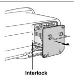
4. Insert a new lamp housing until the lamp housing is plugged into the socket.
