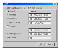
An IP address can be automatically assigned to this projector by your DHCP server. If your network does not automatically assign IP address, ask your network administrator for an address, and then register it manually.
