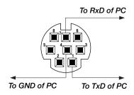
NOTE: Pins 2, 3, 5, 6 and 8 are used inside the projector.
