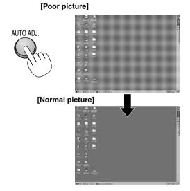
Press the Auto Adjust button to fine-tune the computer image or to remove any vertical banding that might appear and to reduce video noise, dot interference or cross talk (this is evident when part of your image appears to be shimmering). This function adjusts the clock frequencies that eliminate the horizontal banding in the image. This function also adjusts the clock phase to reduce video noise, dot interference or cross talk. (This is evident when part of your image appears to be shimmering.)
