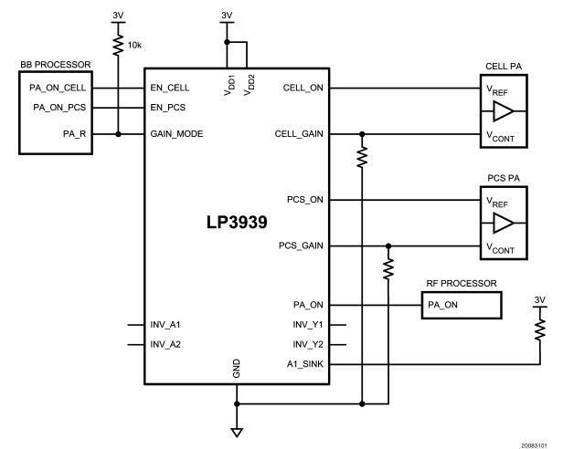
Note: This application circuit shows the connection interface to a typical Skyworks PA. Connections to other PA vendors may vary slightly.
