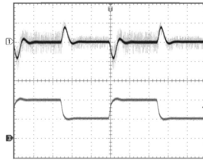
1.28MHz, 8.5V Application Boost Load Step
