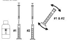
Add 0.5 mL of HI 93738D-0 Reagent D to each cylinder (#1 & #2), close them and invert several times to mix. Cylinder #2 is the sample.
