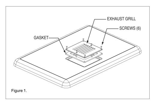
2. Install the Outdoor Vent Kit, (P/N 460424), as shown in Figure 2. Make sure the holes in the gasket, metal flange of the main vent assembly, and heater cover are aligned before securing into place using the six (6) screws provided in the Outdoor Vent Kit.
