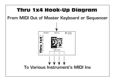
Out of the instrument or sequencer you are "Thruing." Next, connect each of Thru 1x4's MIDI OUTs to the various instrument's MIDI Ins. All of Thru 1x4's MIDI OUTs are identical so it doesn't matter which MIDI OUT is connected to which MIDI In.
