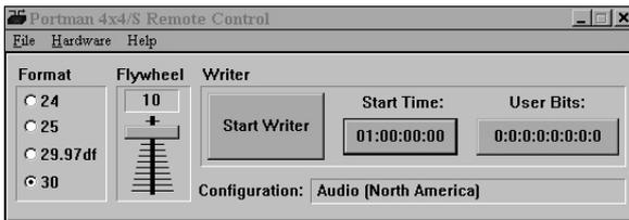
The controls are fairly self-explanatory. Format sets the SMPTE frame rate for the PORTMAN SMPTE generator. Flywheel sets the number of frames the reader/regenerator will automatically advance and correct when receiving either bad or no time code. The Start Writer button starts and stops the SMPTE generator. The Start Time and User Bits buttons allow you to set, respectively, SMPTE start time and user bits.
