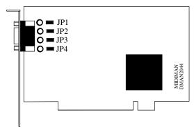
**Input Signal-Level Jumper Positions**
