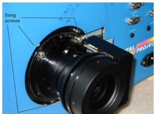
3. Secure the lens using the three cross-head screws.
