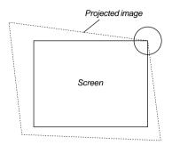
2. Pick up any one of the corners and align the corner of the screen with the one of the image.
