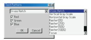
Press to display the test pattern. Pressing this button sequentially selects 11 test patterns for each red, green and blue.
