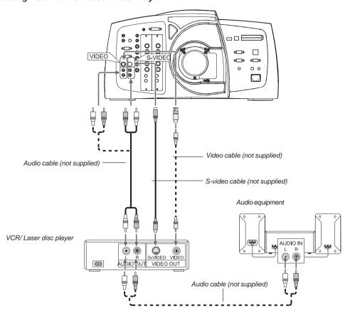
Use common RCA cables (not provided) to connect your VCR, laser disc player or document camera to your projector. To make these connections, simply:
