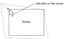
5. Do the above step 4 for the other two corners so that the projected area becomes smaller than the screen.
