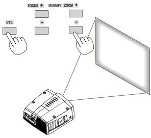
(3) Press and hold the CTL button and press the FOCUS + or button to obtain the best focus. You can also adjust the focus by using the FOCUS + or - button on the projector cabinet.
