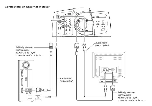
You can connect a separate, external monitor to your projector to simultaneously view on a monitor the RGB analog image you're projecting. To do so:
