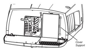
3. Loosen the two screws securing the lamp module until the screws go into a freewheeling condition. The two screws are not removable.
