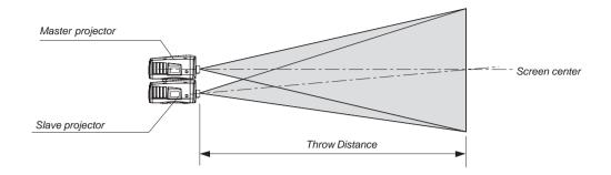
Refer to the table of throw distances in chapter 2, and ensure that the distance between the projectors and the screen is in the middle part of the recommended range for both lenses.
