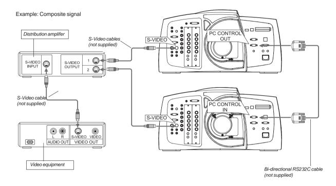
NOTE: Connect a commercially available distribution amplifier to both the master and the slave projectors to distribute signal to two outputs of the master and the slave projectors.
