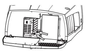
4. Pull the lamp module to the right, then to the rear to remove it from the projector.
