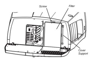
If the filter is severely clogged, or damaged, then it should be replaced.
