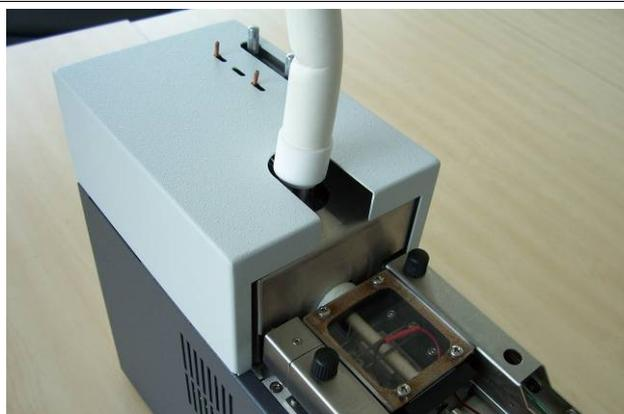
Check the tube receivers to ensure the white PTFE frits are present in both sample and split tube sides.
