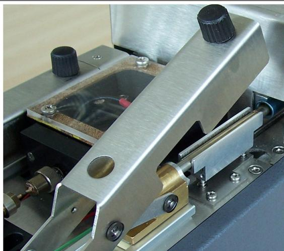
Replace the heated valve surround and secure with the 2 screws removed in the first step
