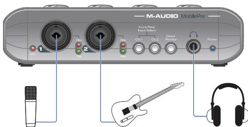
Microphones are connected to either of the combination inputs on the front panel using standard XLR microphone cables.
