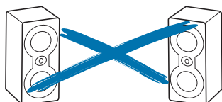
Figure 7: Angled alignment with "toe-in"—Not Recommended
