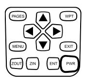
points using the WPT key. The PWR key turns the unit on and off. Pressing it once while the unit is operating turns on the screen's backlight. To prevent an accidental shutdown, you must hold the PWR key down for a few seconds in order to turn the unit off.
