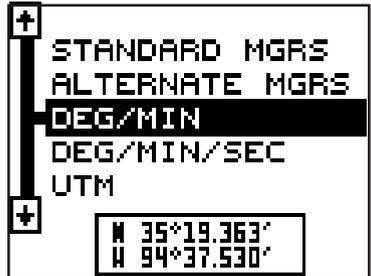
The GlobalNav 310 can show the position in degrees, minutes, and thousandths of a minute (36 28.700') or degrees, minutes, seconds, and tenths of a second (36 28' 40.9"). It can also show position in UTM's (Universal Transverse Mercator) projection, British, Irish, and Military Grid systems.
