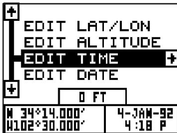
Once the GlobalNav 310 finds and locks on to three satellites, it stops flashing the numbers on the display. (Note: Altitude will still flash until the unit locks on to the fourth satellite. It takes four satellites to determine altitude.)
