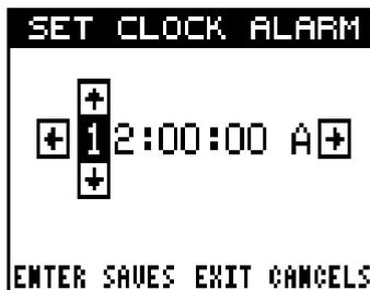
arrow keys until the desired number shows. Continue until the time shown in the display is correct, then press the ENT key. The alarm is now set.
