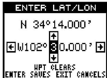
Keep pressing the arrow keys until the latitude and longitude are set to your local position. (Note: This position does not have to be very accurate. If you can get it within one degree of your actual position, that will be fine.) When it's set, press the ENT key. The GlobalNav 310 accepts your entry and returns to the GPS setup menu.
