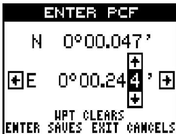
After you've entered the latitude/longitude correction, press the ENT key to accept it. The GlobalNav 310 erases the PCF entry screen and returns to the navigation or mapping screens with the correction factor applied.
