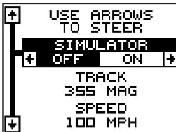
If you simply press the right arrow key, turning the simulator on, the GlobalNav 310 will start from your present position and follow a track of 355° at 100 miles per hour.
