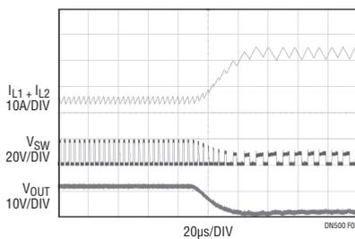
**Figure 3. Short-Circuit Event for the Converter in Figure 1**
