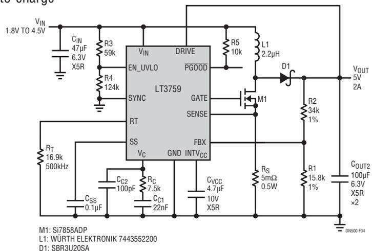
**Figure 4. Boost Converter Produces 5V/2A Output from 1.8V to 4.5V Input**
