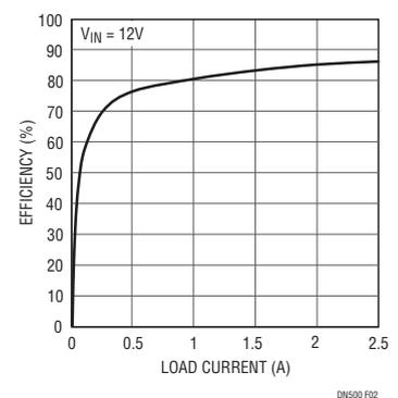
Figure 2. Efficiency for the Converter in Figure 1
