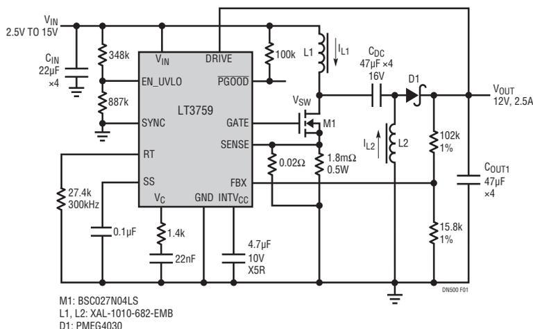
Figure 1. SEPIC Converter Produces 12V Output from 2.5V to 15V Inputs
