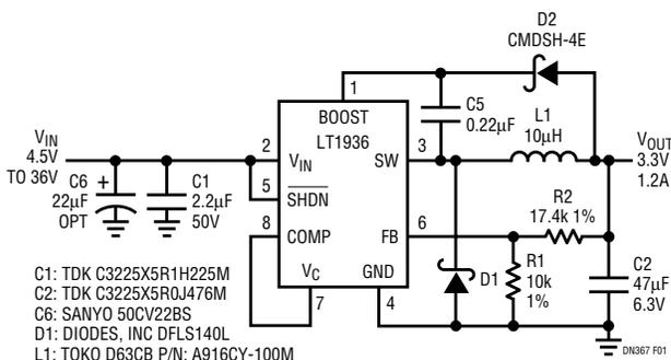
**Figure 1. Typical Application of LT1936 Accepts 4.5V to 36V and Produces 3.3V/1.2A**
