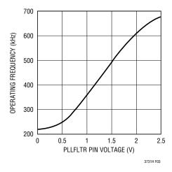
Figure 3. Operating Frequency vs V<sub>PLLFLTR</sub>
