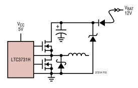
Figure 10. Automotive Application Protection
