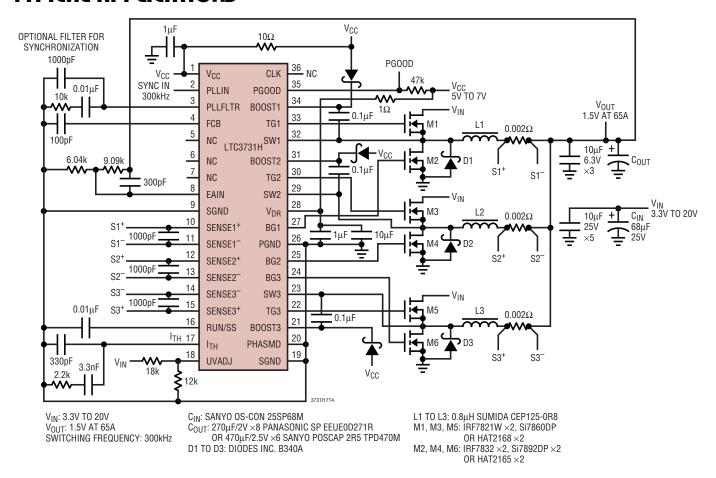
Figure 14. 3-Phase 65A Power Supply
