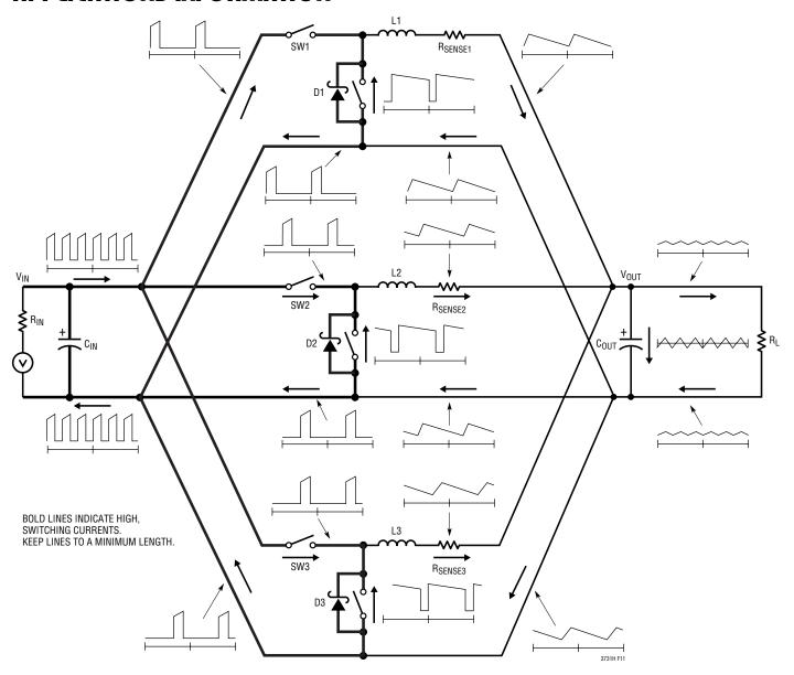
Figure 11. Branch Current Waveforms
