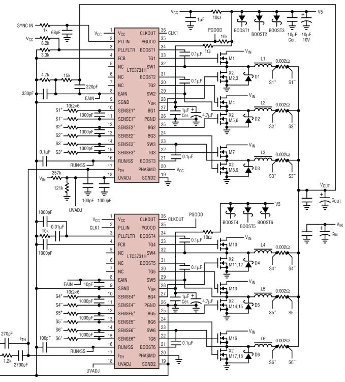
NOTES: V5: 5V TO 7V  $V_{1N}\text{: 10V TO 14V; }V_{OUT}\text{: 2.5V/100A} \\ \text{SWITCHING FREQUENCY: 500kHz (V5 = 5V)}$
