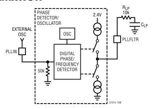
Figure 9. Phase-Locked Loop Block Diagram
