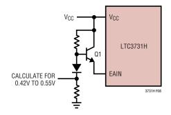
Figure 8. Foldback Current Elimination
