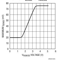
Maximum Current Sense Threshold vs Duty Factor
