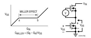
Figure 5. Gate Charge Characteristic
