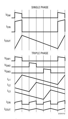
Figure 13. Single and Polyphase Current Waveforms
