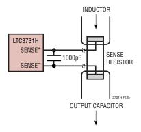
Figure 12. Kelvin Sensing R<sub>SENSE</sub>
