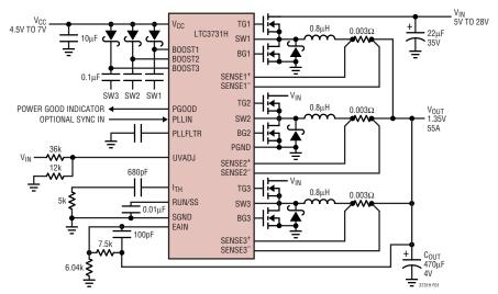
Figure 1. High Current Triple Phase Step-Down Converter
