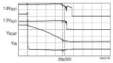
Figure 2. Supercapacitor Backup Time Supporting a 20W Load
