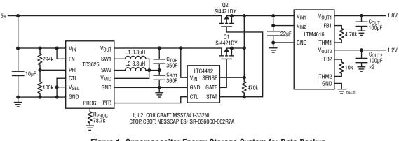
Figure 1. Supercapacitor Energy Storage System for Data Backup
