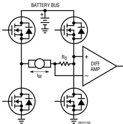
Figure 3. Limited Performance H-Bridge Current Monitor
