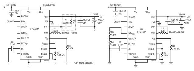
Figure 2. Buck-Boost Converter Produces 12V<sub>OUT</sub> at 5A from a 5V to 20V Input Range
