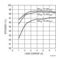
Figure 3. Buck Converter Produces a 24V Output with 168W Capability
