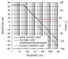
Figure 8. Voltage loop Bode design with current closed loop having 0,-1 shape
