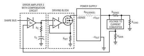
Figure 5. Current loop functional block diagram
