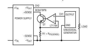
Figure 1. Power supply closed-loop Bode plot measurement block diagram
