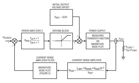
Figure 6. Current loop control block diagram
