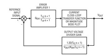
Figure 7. Voltage loop control block diagram
