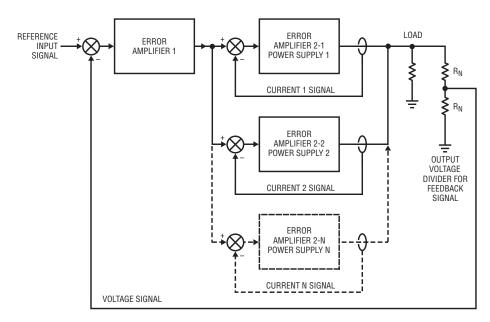
Figure 2. Power system control loop
