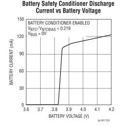
Figure 1. The Battery Conditioner Protects the Battery by Releasing Energy to Lower the Battery Voltage when the Battery Is Hot. The Battery Conditioner Discharge Current Varies with Battery Voltage, as Shown Here.
