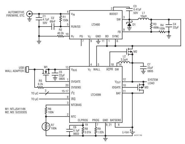
Figure 3. A single IC, the LTC4099, Efficiently Manages Power from Three Sources: the USB, a Li-Ion Battery and a Stepped-Down High Voltage Source. Its Efficient Battery Charger Uses the Bat-Track Feature to Minimize Power Losses When Charging the Battery.
