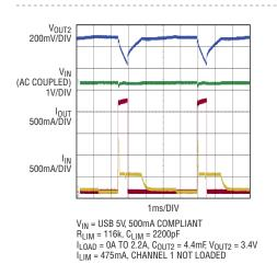
Figure 2. Operation of the GSM modem power supply showing bursts of current beyond the input current limit and quick charging of the supercap on  $V_{OUT2}$ . Note the stability of  $V_{IN}$ .
