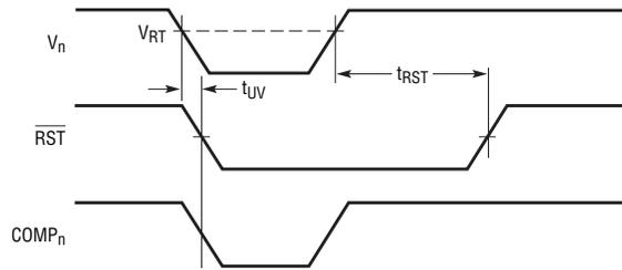
**Figure 5.  $\overline{RST}$  timing diagram**
