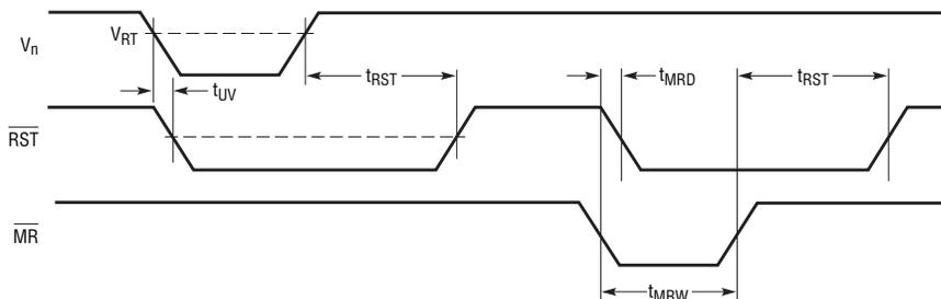
Figure 8.  $\overline{MR}$  timing diagram
