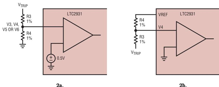
Figure 2. Using a resistive divider to set the voltage trip point
