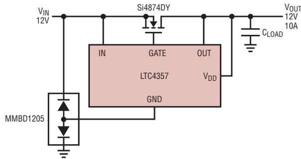
**Figure 3. -12V Reverse input protection blocks reverse input voltage to the load**
