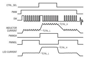
Figure 2. LED current PWM and CTRL\_SEL dimming
