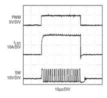
Figure 9. 0A to 20A switched cathode PWM dimming
