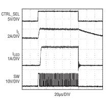
Figure 7. 0A to 2A current limited shunted output PWM dimming
