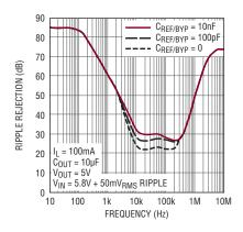
Figure 4. LT3050 ripple rejection
