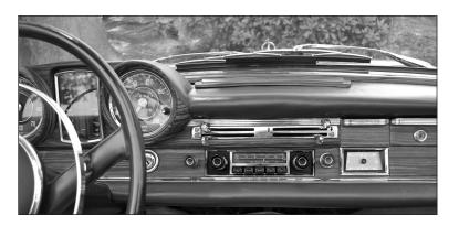
Figure 1. Old school dashboard; one passive antenna for AM/FM reception
