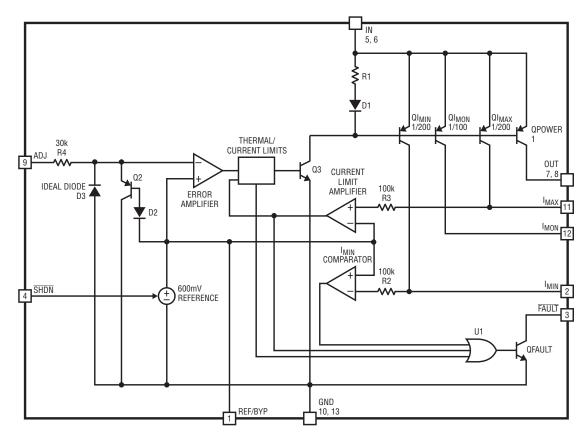
Figure 5. LT3050 block diagram
