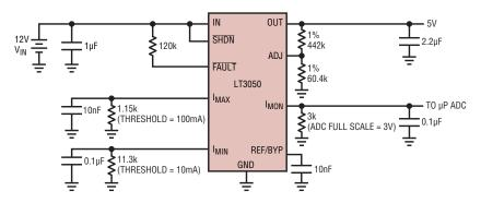
Figure 6. LT3050 active antenna supply circuit
